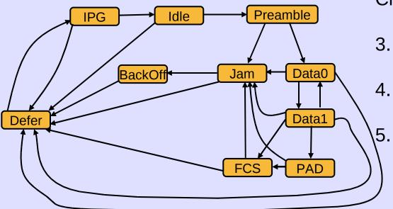
Transmit Module In Ethernet MAC (self-loop on each state not shown)
